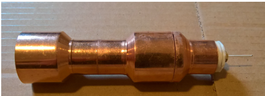
The scope with the front sealed and the sight element fitted.
