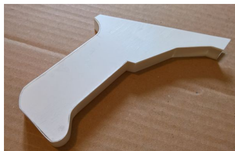
The grip body with the end points of the covering strip marked on and with the strip glued in place.
