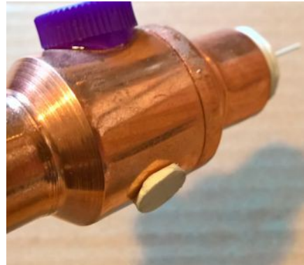
The ribbed caps fitted to the top and left of the scope and disc glued to the right underside.
