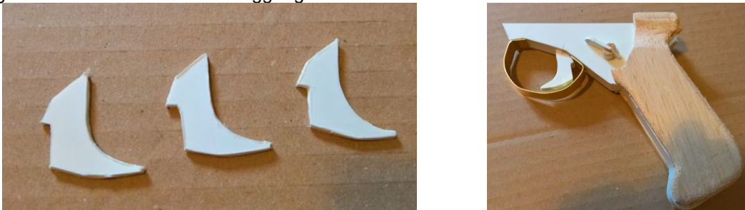
The three identical pieces of the trigger and the trigger and guard glued to the grips.
