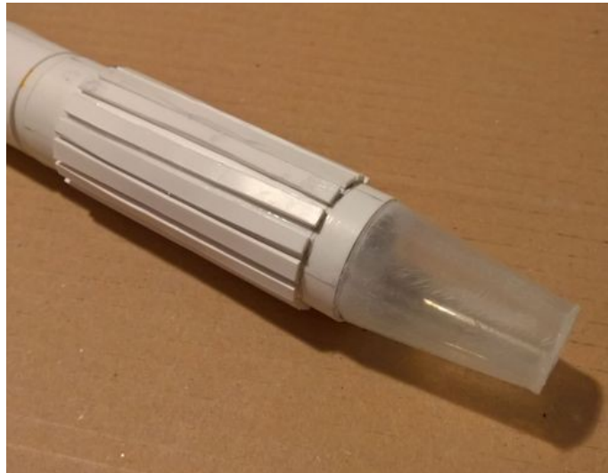
The ribs fitted around the body.
