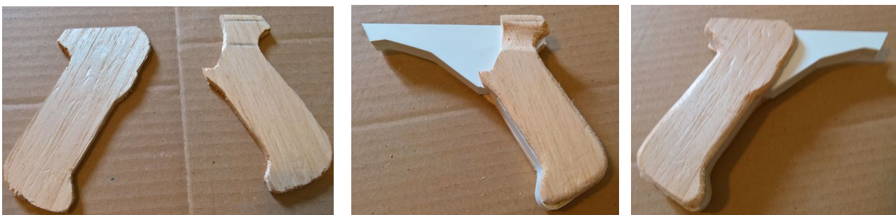
Left to right: The basic pieces of the grips plus the sanded left and right grips glued in place. Note the curved channel sanded into the left grip.
