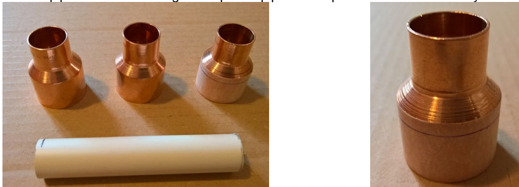
The three reducers and length of pipe used for the scope, plus a close up of the reducer marked for cutting. Masking tape has been wrapped around it to make drawing on it easier.
