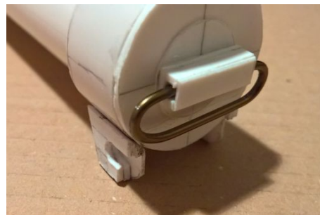
The swivel, channel and cover and the completed swivel assembly fitted to the end cap.
