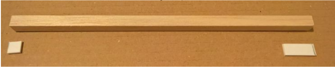
The body of the scope mount plus the two supporting pieces.
