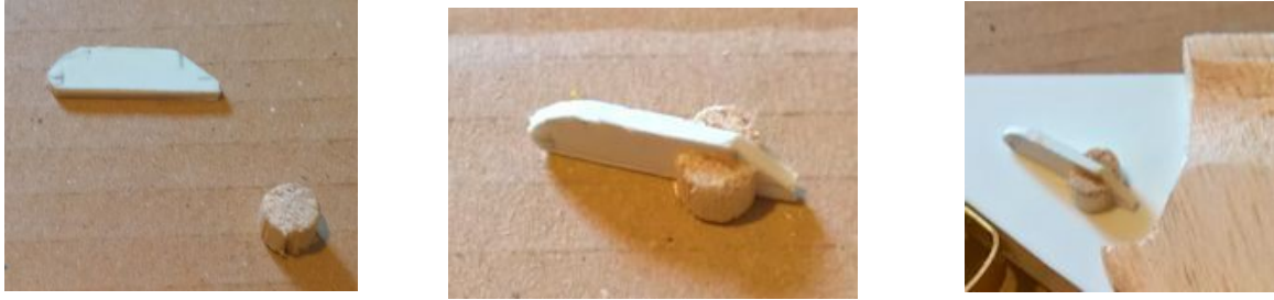
Left to right: The parts of the selector, the assembled selector and the selector glued to the grip body.
