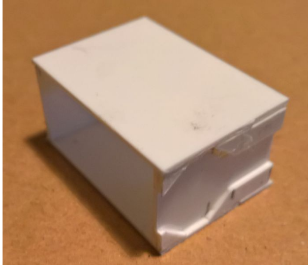
The hollow magazine showing the four details in the corners and with the top/bottom detail pattern added.
