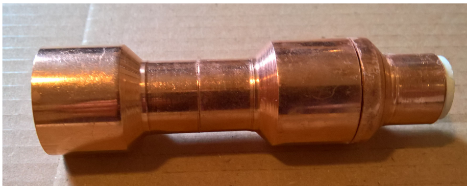
The basic body of the scope. Note the protruding plastic pipe at the front.
