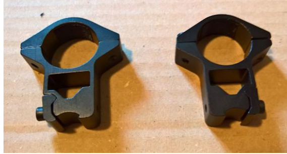
25mm scope mounts. This type is too tall and needs cutting down.
