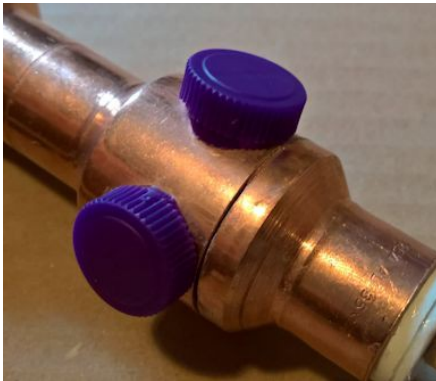
The ribbed caps fitted to the top and left of the scope and disc glued to the right underside.
